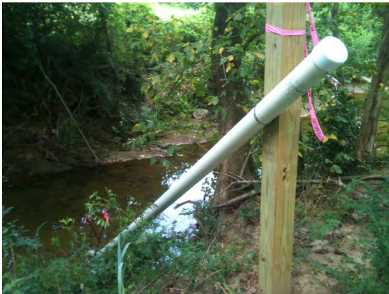
Hydrolab DS5 Sonde in Parkerson Mill Creek – Representative of Typical Deployment
